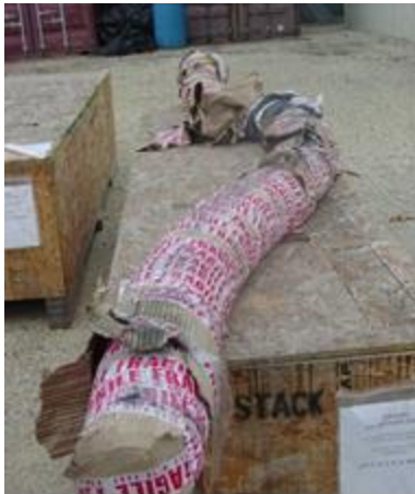
Figure 14: Component Wrapping at Destination Indicating Shipping Damage
