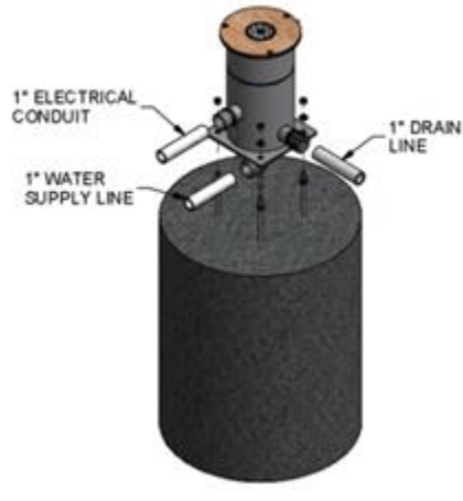
Figure 19: Luminary Cannister Installation
