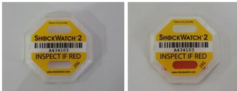
Figure 15: Shock Watch Sticker OK (Left) vs. Not OK (Right)
