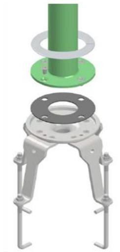
Figure 33: Feature Installation on PlayPHASE Base
