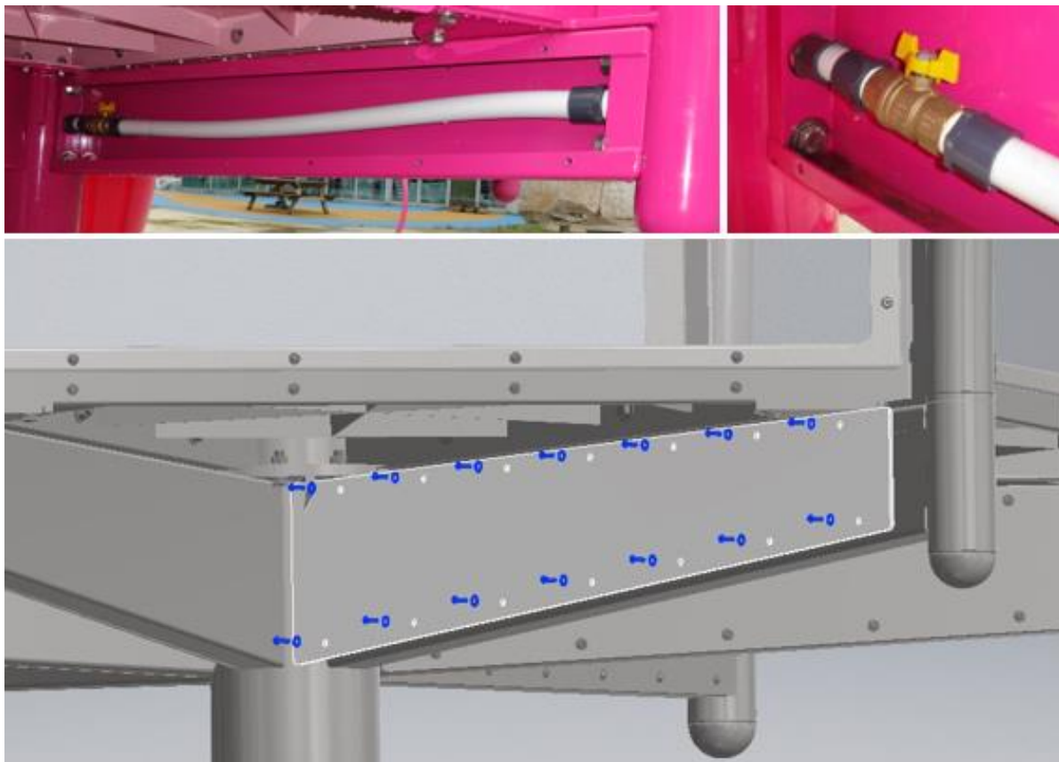
Figure 25: Floating Column Water Distribution
