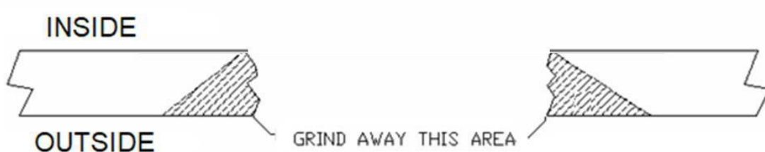
Figure 28: Grind Away Repair Area
