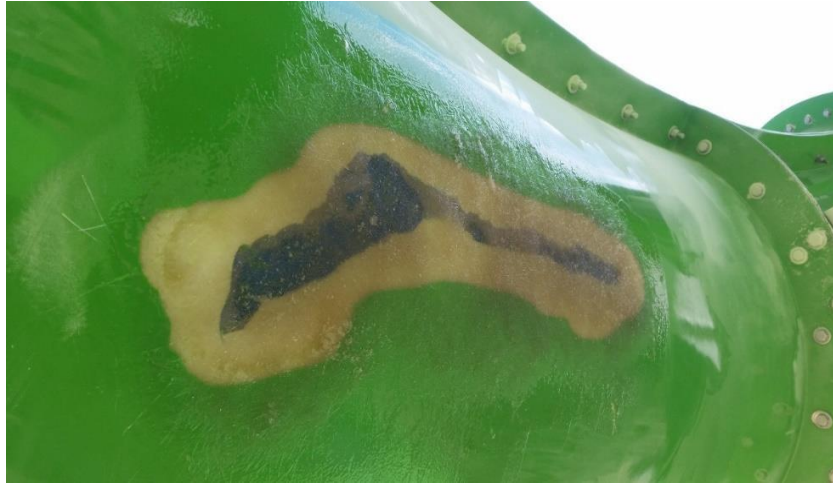
Figure 39: Cured Fiberglass Repair, Outside
