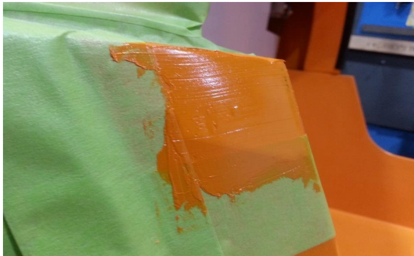
Figure 43: Applying Gelcoat Putty
