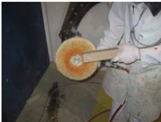
Figure 65: Apply Buffing Compound to Pad
