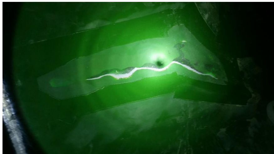
Figure 46: Sanded and Cleaned Putty on Fiberglass Repair, Inside
