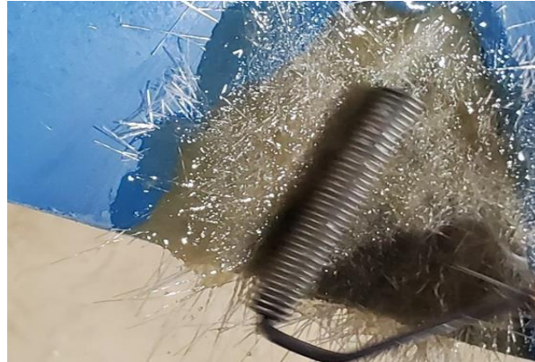
Figure 37: Smooth Out Air Bubbles with Metal Roller
