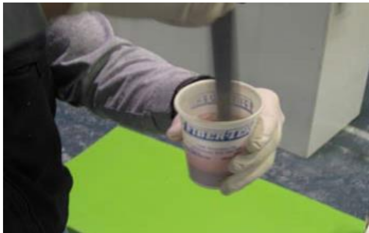
Figure 49: Mix Gelcoat and Pro Patch
