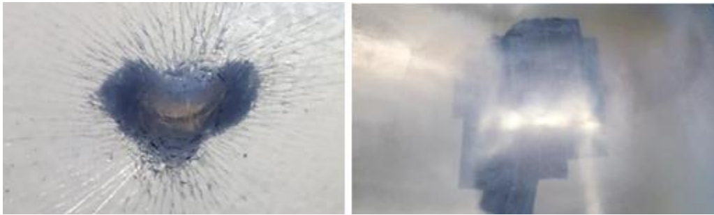
Figure 25: Translucent Inside Damage and Buffed Inside Repair, Before and After
