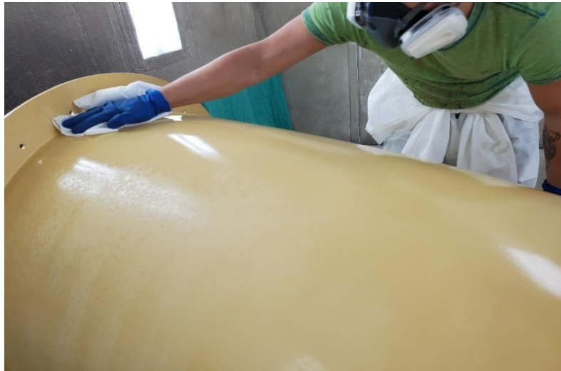
Figure 71: Wipe Sanded FRP with Wax and Grease Remover
