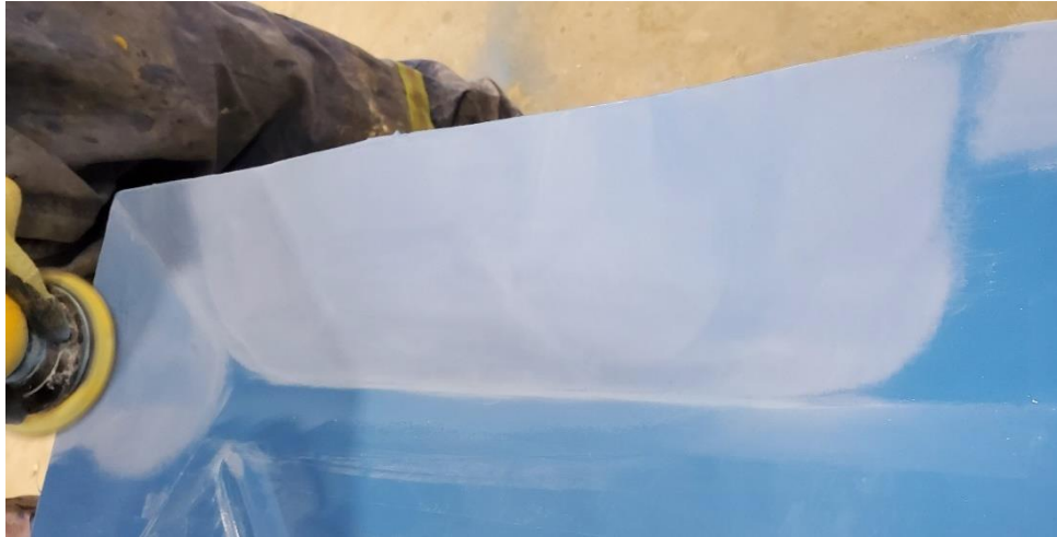
Figure 55: Sand with 400 to 600 grit Sandpaper
