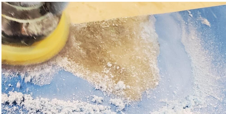
Figure 40: Sanding Fiberglass Repair
