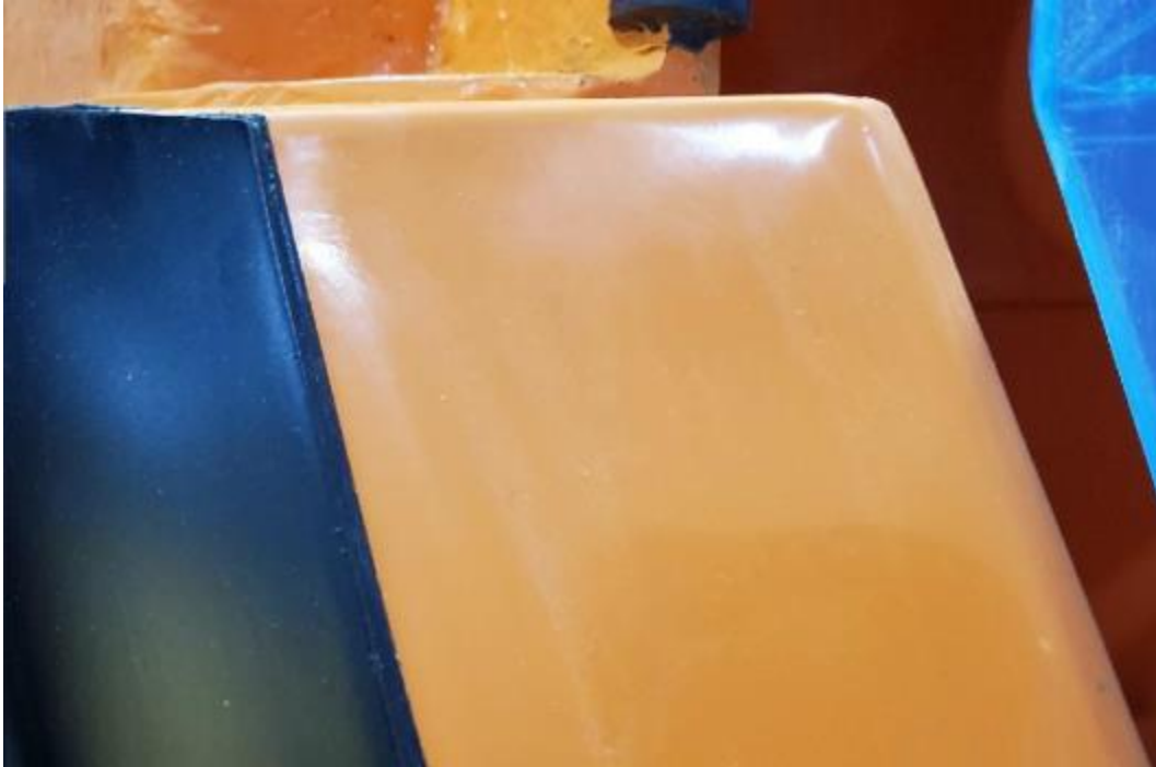
Figure 67: Buffed Small Putty Repair
