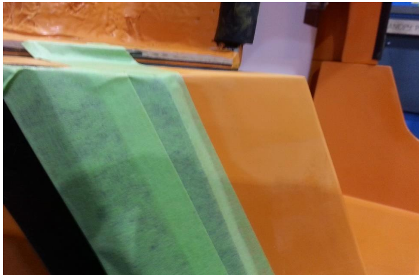
Figure 44: Sanded Gelcoat Putty Repair
