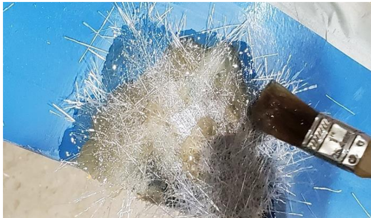
Figure 36: Use Paint Brush to Soak Fiberglass with Resin
