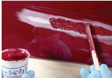
Figure 26: Vertical Surface Repairs
