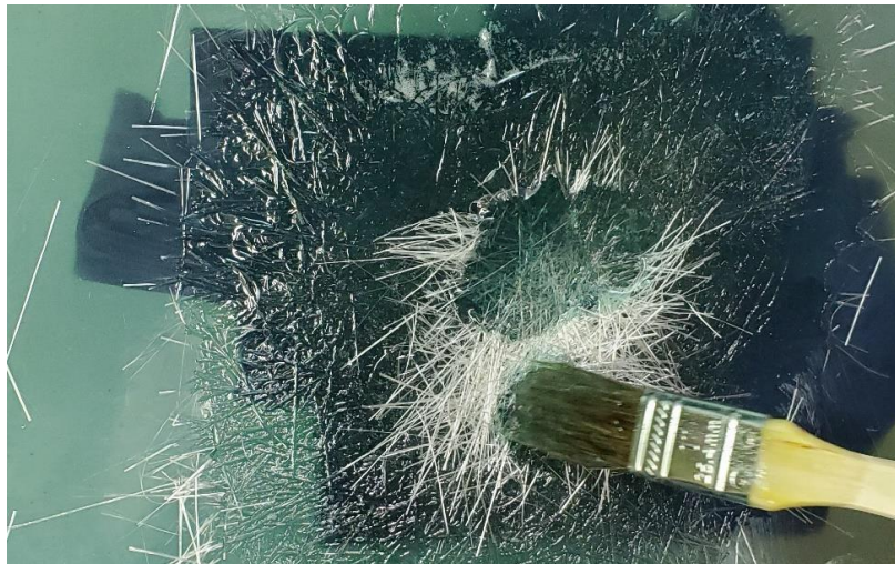
Figure 38: Soak Fiberglass with Paint Brush
