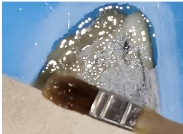
Figure 35: Wet Repair Area with Resin Mixture
